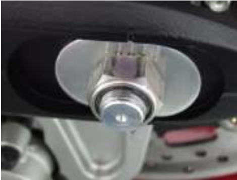
Recessed oval shaped belt tension washer
