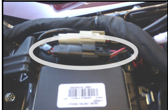
Harness Connector Location—on top of ECM
